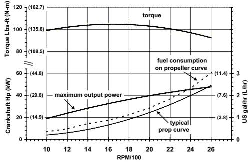
Westerbeke recommends a propeller that will allow the engine to turn 2600 rpm underway at full throttle. Output is according to ISO 8665/3046. Fuel density 0.840 kg/L at 15 °C. Output includes +/- 5% tolerance.
